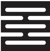
1/8" x 1" Oblong Side Staggered 1/4" Centers 43% Open
